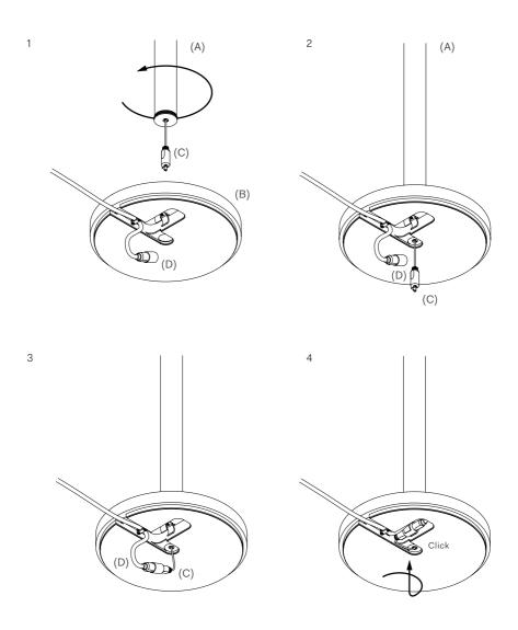
1 Feed the Connector (E) through the central hole of the Head.
