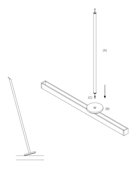
1 Feed the Connector (C) through the central hole of the Base (B) and screw the Glass Tube (A) to the Base (B).
